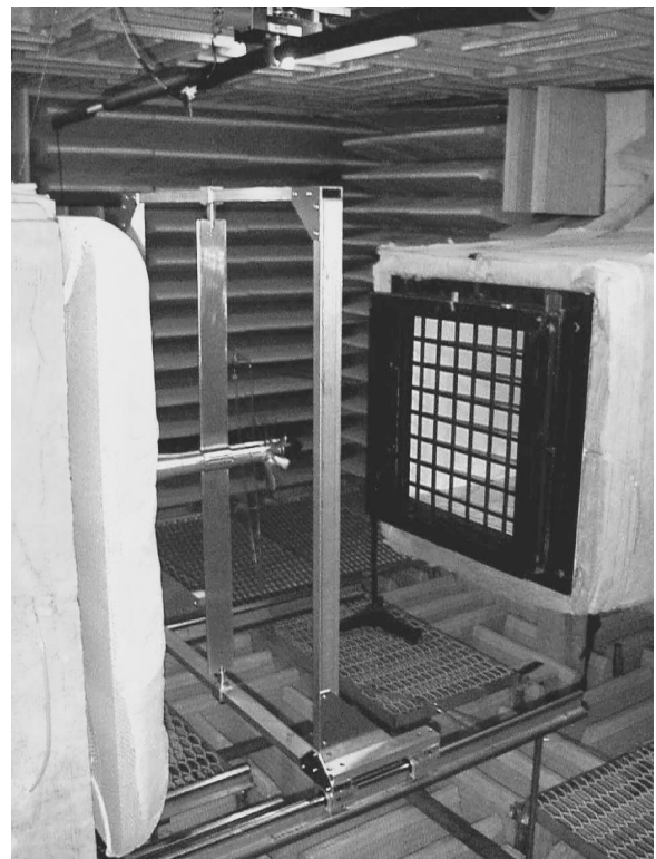
Fig. 3 Propeller/stator test rig mounted in AWT.
